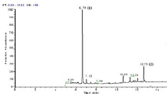
**Fig. 1** Chromatograms of air composition from a workplace obtained by GC/MS. The peaks were identified as nicotine (1) and atrazine (2)
