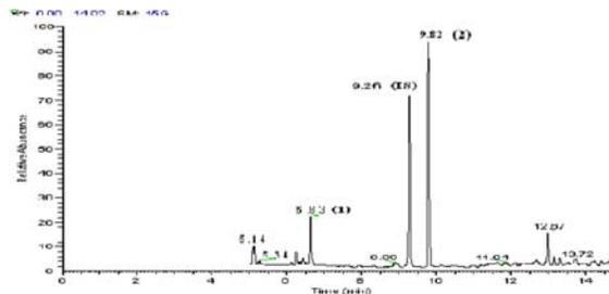
**Fig. 2** Chromatogram of a urine sample from an exposed worker obtained by GC/MS using the SIM technique. The peaks were identified as nicotine (1), diphenylamine (IS), and cotinine (2)
